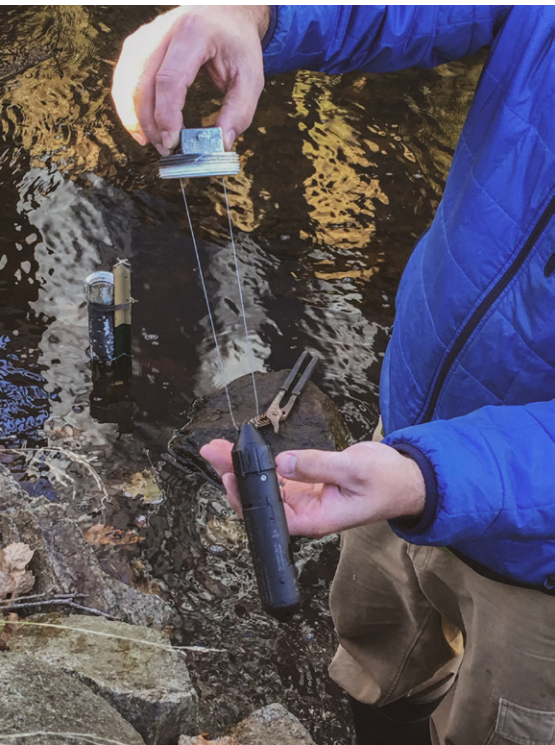
Installing HOB0 water level pressure transducers in stream bed below Norwood Ave.
