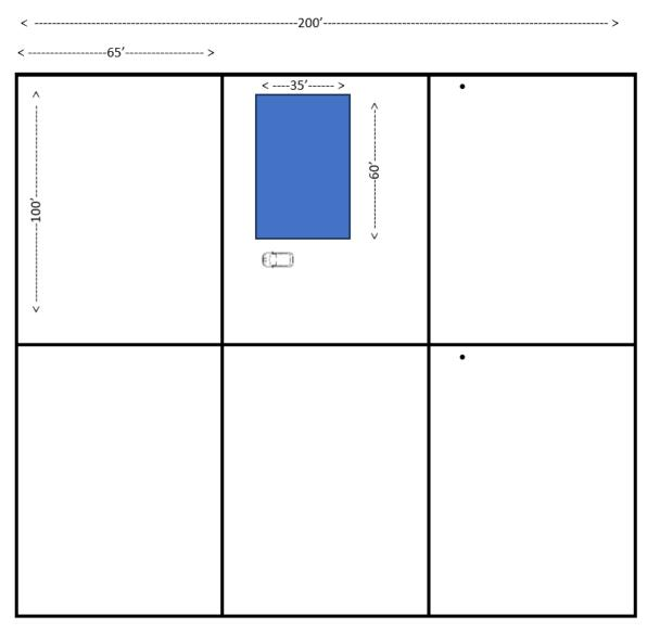
The building footprint in blue is 35 Ft X 60 Ft, or 2,100 SF. This diagram shows a car parked in the back yard. Setbacks are 5 Ft on the front and 10 Ft on the side. There is space for a 15-foot-wide driveway on the right. Lot coverage would be less than 33%. This would provide a single-story house of about 1,800 net SF. These lot dimensions comply with current zoning.
