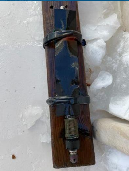
Figure 13: Photo of the tide gauge deployed during Manchester study
