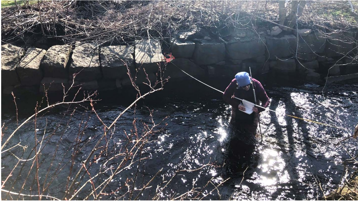
Photo 2: Sawmill Brook Stream Discharge Measuring. Stream velocity in feet/second is measured at discrete intervals across the channel. Stream discharge in cubic feet per second is obtained by multiplying the area for each interval.
