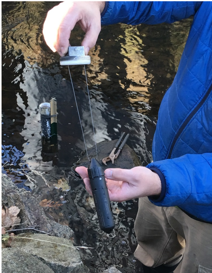
Photo 3: Method to deploy HOB0 water level pressure transducers in stream bed below Norwood Ave. The PVC casing attached to fence post is shown to the left. The PVC was painted black to deter vandalism.
