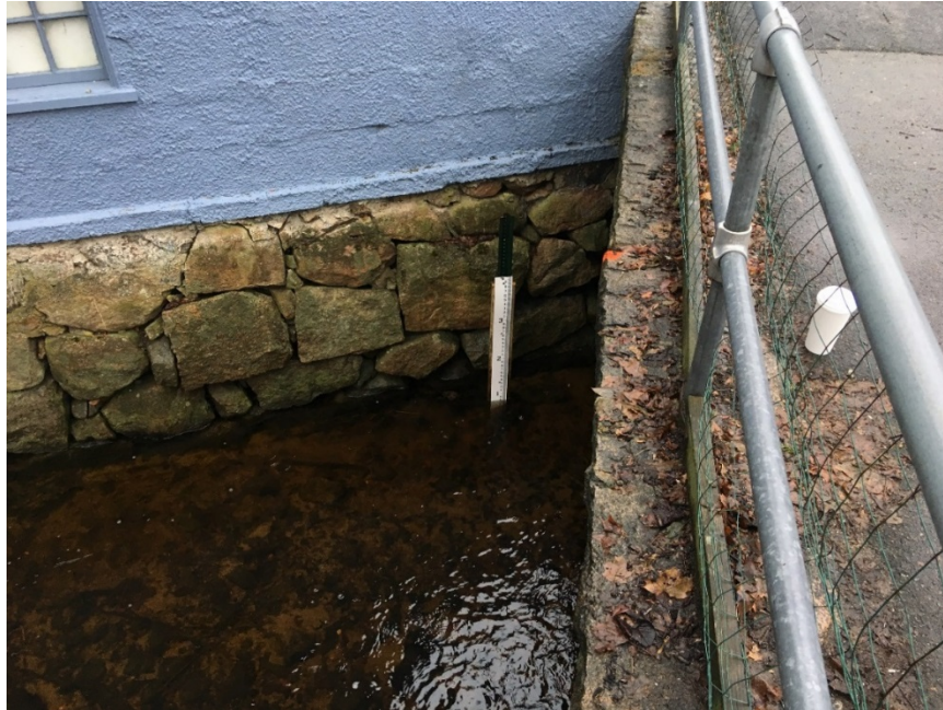
Photo 8: The downstream side of the Norwood Avenue is shown here. Gage A is installed on a heavy-duty fence post, pounded deep into the stream bottom. Volunteers took weekly depth to water measurements at the headwall bench mark location, indicated by the orange mark at the edge of the pavement.
